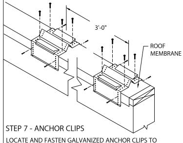
THE WALL AT 3'-0" O.C. WITH PROVIDED FASTENERS (SEE DETAIL A)
