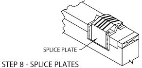
PLACE SPLICE PLATE ONTO ANCHOR CLIPS AT SPLICE JOINTS, 12'-0" O.C.
