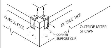
STEP 1 - CORNER SUPPORT CLIPS LOCATE AND FASTEN GALVANIZED CORNER SUPPORT CLIPS TO THE WALL.
