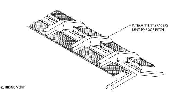
THE RIDGE VENT IS MANUFACTURED TO BEND TO ACCOMMODATE 3/12 TO 12/12 ROOF PITCHES. SIMPLY SET RIDGE VENT ON ROOF AND BEND SPACERS TO THE CORRECT PITCH.
