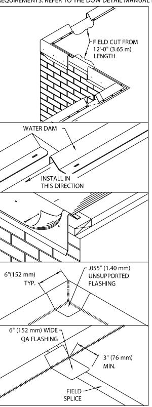
1. LOCATE AND INSTALL MITERS, NAILING THROUGH PRE-SLOTTED FASTENING HOLES ON TOP FLANGE ONLY. DETERMINE AND IDENTIFY LOCATION OF SCUPPERS. DO NOT INSTALL SCUPPERS AT THIS TIME. LEAVE GAP OF 14 1/2" (368 mm) INCHES FOR SCUPPER LOCATIONS. THEN INSTALL THE 12'-0" (3.65 m) SECTIONS OF WATER DAM FROM RIGHT TO LEFT (AS SEEN FROM ROOF TOP) BY NAILING THROUGH SLOTTED HOLES PROVIDED PER JOB REQUIREMENTS. FIELD CUT SECTIONS AS NECESSARY. LAP WATER DAM JOINTS 1" (25 mm).
