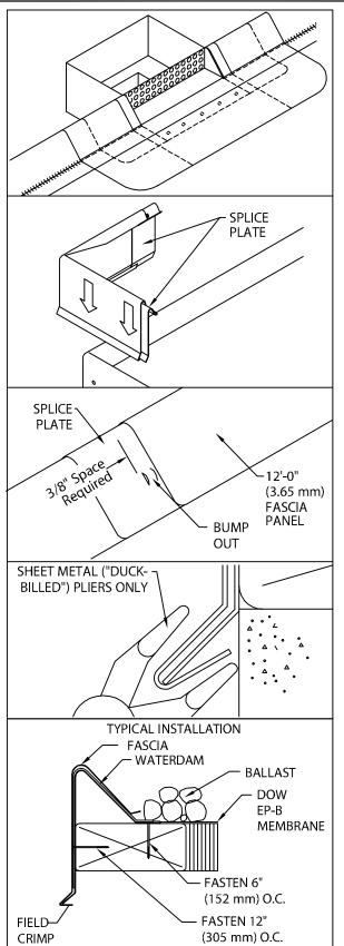
5. INSTALL SPILLOUT OR DOWNSPOUT SCUPPERS (IF APPLICABLE) AT PRE-DETERMINED LOCATIONS USING PROVIDED NAILS.
