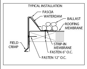
7. COMPLETE INSTALLATION BY PLACING BALLAST (IF REQUIRED), FOLLOWING ROOF MEMBRANE MANUFACTURERS' RECOMMENDATIONS.
