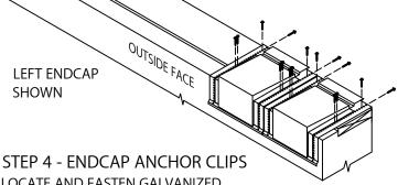
LOCATE AND FASTEN GALVANIZED ANCHOR CLIPS TO WALL WITH PROVIDED FASTENERS FOR SUBSTRATE (SEE DETAIL A).
