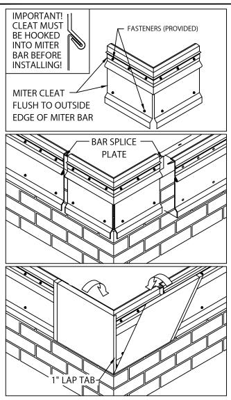
5. MITER BAR & MITER CLEAT INSTALLATION HOOK MITER CLEAT PIECES TO MITER BAR. FLUSH ENDS OF MITER CLEAT PIECE AND MITER BAR. INSTALL MITER ASSEMBLY WITH ONE ANCHOR BAR SPLICE PLATE UNDER EACH END OF MITER BAR. FASTEN THE MITER BAR USING PROVIDED FASTENERS AND DRIVE BITS. NEXT LOCATE AND INSTALL THE SPILLOUTS AND SCUPPERS WITH FASTENERS AND SPLICE PLATES.
