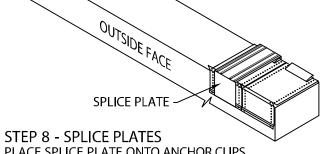
PLACE SPLICE PLATE ONTO ANCHOR CLIPS AT SPLICE JOINTS, 12'-0" (3.65 m) O.C.
