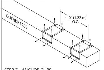
STEP 7 - ANCHOR CLIPS LOCATE OVER MEMBRANE AND FASTEN **GALVANIZED ANCHOR CLIPS TO WALL** AT 4'-0" (1.22 m) CENTER WITH PROVIDED FASTENERS AS SHOWN IN DETAIL A.
