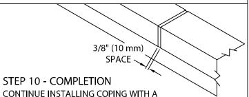
CONTINUE INSTALLING COPING WITH A 3/8" (10 mm) SPACE AT SPLICE JOINTS TO ALLOW FOR THERMAL EXPANSION. FIELD CUT WHERE NECESSARY USING FINE TOOTH HACKSAW OR SNIPS. NOTE: REMOVE PROTECTIVE FILM IMMEDIATELY.
