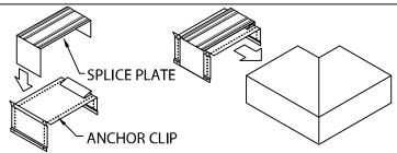
STEP 2 - MITER SPLICE PLATES & ANCHOR CLIPS POSITION THE SPLICE PLATE IN THE CENTER OF THE ANCHOR CLIP. INSTALL THE SPLICE PLATE AND ANCHOR CLIP ASSEMBLY HALFWAY INTO EACH END OF THE CORNER AS SHOWN
