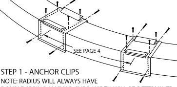
DOUBLE SPRING ANCHOR CLIPS. WIDTH WILL BE DETERMINED BY RADIUS SIZE AND MATERIAL.
