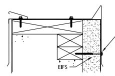
If using an EIFS system, fasten through face w/ fastener of proper length to penetrate nailer
