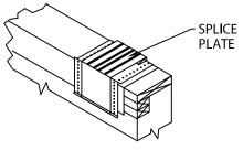
STEP 8 - SPLICE PLATES PLACE SPLICE PLATE ONTO ANCHOR CLIPS AT SPLICE JOINTS, 12'-0" (3.65 m) O.C. NOTE: REMOVE RELEASE PAPER FROM SEALANT STRIPS.
