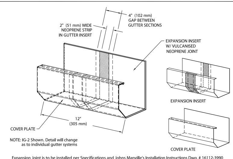
Expansion Joint is to be installed per Specifications and Johns Manville's Installation Instructions Dwg. # 16112-3990
