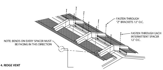
SET RIDGE VENT IN PLACE CENTERED OVER RIDGE OPENING. THE BENDS ON TOP OF THE SPACER MUST ALL BE FACING AWAY FROM THE END OF THE ROOF. FASTEN THROUGH PRE-PUNCHED SLOTTED HOLES IN INTERMITTENT SPACERS AT 12" O.C. WITH APPROPRIATE FASTENERS. ALSO FASTEN THROUGH PRE-PUNCHED SLOTTED HOLES IN "Z" BRACKETS 12" O.C.. LAP "Z'S" 1".
