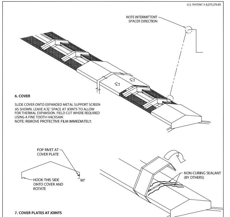
APPLY A GENEROUS BEAD OF NON-CURING SEALANT (BY OTHERS) TO EACH SIDE OF JOINT. HOOK COVER PLATE ONTO COVER AT JOINTS AND ROTATE INTO PLACE. POP RIVET INTO COVER PLATE AT ONE SIDE OF THE JOINT (FASTEN SIDE WHICH HAS 90° DRIP ANGLE). THIS WILL PREVENT MIGRATION.
