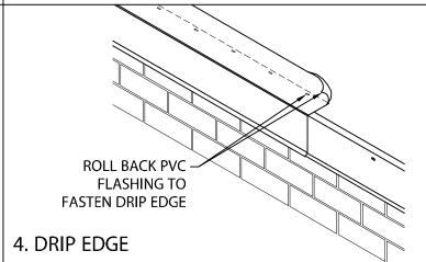
ROLL BACK PVC FLASHING TO EXPOSE FASTENING SLOTS AND FASTEN THRU PRE-SLOTTED HOLES 6" WITH PROVIDED NAILS.
