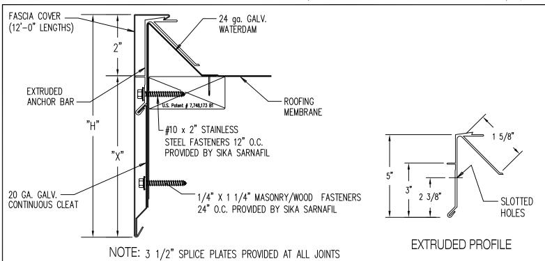
Fascia is to be installed per Specifications and Sika Sarnafil's Installation Instructions Dwg. # 14110-2842
