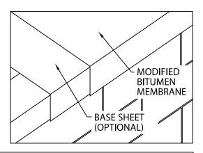
NOTE: Flex may require a sacrificial flashing strip. (Refer to drawing 2A & 2B). Please check with Flex prior to installation.
