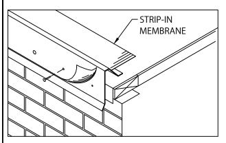
3. POSITION STRIP-IN MEMBRANE OVER AND DOWN WATERDAM FACE APPROXIMATELY 1" BELOW RAISED FASTENING HOLES (PROVIDED). TAKE CARE TO AVOID BRIDGING OF MEMBRANE. LOCATE AND FASTEN MEMBRANE AT 12" O.C. THROUGH ALL RAISED HOLES ON OUTSIDE FACE USING PROVIDED FASTENERS.
