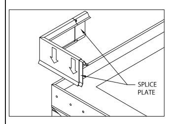
4. INSTALL MITER COVERS FIRST, INSERT ONE SPLICE PLATE UNDER EACH END OF MITER COVER. ALLOW 3/8" SPACE BETWEEN ENDS OF ADJOINING FASCIA PANELS. INSTALL MITER COVERS BY PUSHING DOWNWARD UNTIL COVER IS ENGAGED ALONG ENTIRE MITER. CRIMP ENTIRE DRIP EDGE OF EACH MITER COVER AS SHOWN IN STEP #6.
