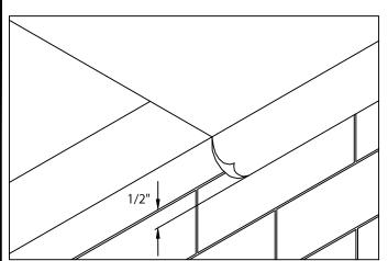
1. POSITION MEMBRANE OVER THE ROOF EDGE AND DOWN OUTSIDE FACE OF WALL, COVERING TREATED WOOD NAILER(S) COMPLETELY. ALLOW 1/2" EXCESS MEMBRANE.
