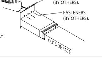
STEP 9 - ENDWALL FLASHING SPLICE PLATE VERSION STEPS 9 - 10 NOTE: WITH THE ENDWALL FLASH SPLICE PLATE VERSION THERE IS ONE ANCHOR CLIP.
