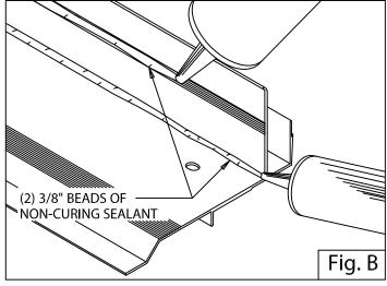
3. Miter & Scupper Anchor Bar (Preparation)
