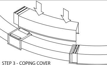
NOTE: 4'-0" O.C. SHOWN REMOVE RELEASE PAPER FROM RIGHT TWO FACTORY APPLIED SEALANT STRIPS ON THE SPLICE PLATE IN THE COPING SECTION.
