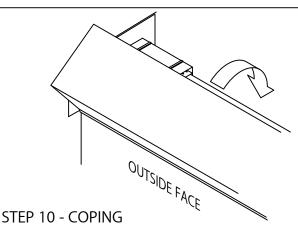
HOOK OUTSIDE FACE OF COPING OVER THE ANCHOR CLIP/ENDWALL FLASHING AND ROTATE INTO PLACE. ENGAGE REAR LEG ONTO ANCHOR CLIP BY PRESSING DOWNWARD UNTIL SNAP LOCK OCCURS.
