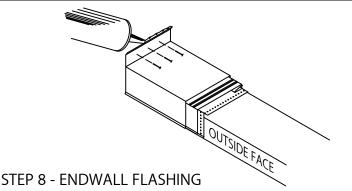
FASTEN TO WALL USING APPROPRIATE FASTENERS AS SHOWN. APPLY NON-CURING SEALANT (BY OTHERS) TO CAULK CUP ATOP 3" FLANGE.
