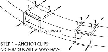
DOUBLE SPRING ANCHOR CLIPS. WIDTH WILL BE DETERMINED BY RADIUS SIZE AND MATERIAL.
