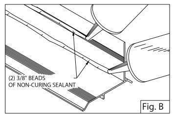
3. Miter & Scupper Anchor Bar (Preparation)
