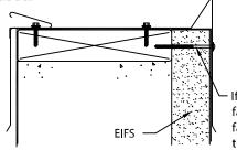
If using an EIFS system, fasten through face w/ fastener of proper length to penetrate nailer
