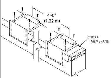
STEP 7 - ANCHOR CLIPS LOCATE AND FASTEN GALVANIZED ANCHOR CLIPS TO WALL AT 4'-0" (1.22 m) CENTERS WITH PROVIDED FASTENERS FOR SUBSTRATE (SEE DETAIL A).
