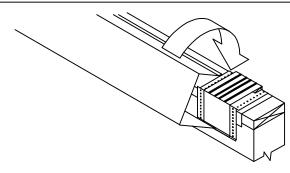
STEP 9 - COPING HOOK OUTSIDE FACE OF COPING OVER THE ANCHOR CLIPS AND ROTATE INTO PLACE. ENGAGE REAR LEG ONTO ANCHOR CLIPS BY PRESSING DOWNWARD UNTIL SNAP LOCK OCCURS.
