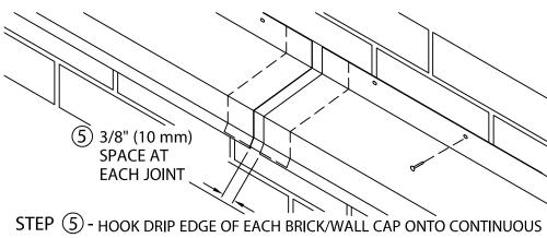
STEP (5) - HOOK DRIP EDGE OF EACH BRICK/WALL CAP ONTO CONTINUOUS CLEAT, ROTATE INTO PLACE, AND FASTEN WITH APPROPRIATE FASTENERS. CONTINUE BY INSTALLING BRICK / WALL CAP SECTIONS AND SPLICE PLATES, ALLOWING A 3/8" (10 mm) SPACE AS SHOWN. FIELD CUT AS NECESSARY.
