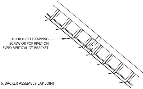
LAP ONE 12'-0" PIECE OF BACKER ASSEMBLY 1" OVER THE PREVIOUS BACKER ASSEMBLY AS SHOWN. FASTEN THE 24 GA. GALV. BACKER OF THE 12'-0' PIECE TO THE 24 GA. GALV. BACKER OF THE USING #8 X  $\frac{1}{2}$ " SELF-DRILLING PAN HEAD FASTENERS. USE 3 FASTENERS FOR "H" DIMENSIONS 12" OR LESS AND 6 FASTENERS FOR "H" DIMENSIONS GREATER THAN 12". FASTENERS CAN BE
