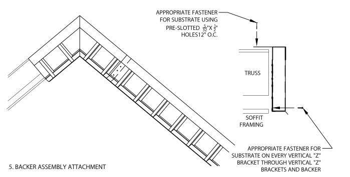
ATTACH THE ROOF FLANGE OF THE BACKER ASSEMBLY TO THE TOP OF THE SHEATHING WITH AN APPROPRIATE FASTENER FOR THE SUBSTRATE USING THE PRE-SLOTTED  $\frac{5}{32}$ " X $\frac{1}{2}$ " HOLES AT 12" O.C. ATTACH THE BACKER ASSEMBLY THROUGH THE VERTICAL "Z" BRACKETS AND BACKER USING APPROPRIATE FASTENER FOR SUBSTRATE ON EVERY VERTICAL "Z" BRACKET.
