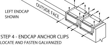
LOCATE AND FASTEN GALVANIZED ANCHOR CLIPS TO WALL WITH PROVIDED FASTENERS FOR SUBSTRATE (SEE DETAIL A).
