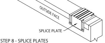
PLACE SPLICE PLATE ONTO ANCHOR CLIPS AT SPLICE JOINTS, 12'-0" O.C.
