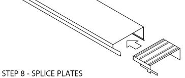
REMOVE RELEASE PAPER FROM TOP OF FACTORY APPLIED SEALANT STRIPS. PLACE SPLICE PLATE HALFWAY INTO ONE END OF 12'-0" LENGTH OF COPING AS SHOWN.
