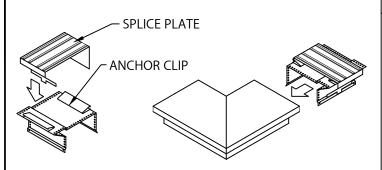
STEP 2 - MITER SPLICE PLATES & ANCHOR CLIPS POSITION THE SPLICE PLATE IN THE CENTER OF THE ANCHOR CLIP. INSTALL THE SPLICE PLATE AND ANCHOR CLIP ASSEMBLY HALFWAY INTO EACH END OF THE CORNER AS SHOWN.
