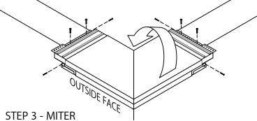
HOOK OUTSIDE FACE OF MITER ASSEMBLY ONTO CORNER CLIP AND ROTATE INTO PLACE. SECURE AT THE EXPOSED EDGE OF THE ANCHOR CLIP AS PER DETAIL A.
