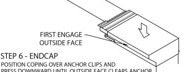
POSITION COPING OVER ANCHOR CLIPS AND PRESS DOWNWARD UNTIL OUTSIDE FACE CLEARS ANCHOR CLIPS. ENGAGE OUTSIDE FACE BY PUSHING DOWNWARD ON FRONT EDGE UNTIL SNAP LOCK OCCURS. THEN ENGAGE INSIDE FACE BY PUSHING DOWNWARD ON BACK EDGE UNTIL SNAP LOCK OCCURS.
