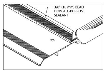
2. Miter & Scupper Anchor Bar (Preparation) Lay miters and spill out scuppers on deck with outside face down. Be sure aluminum anchor bar is clean and free of dirt or dust. Apply a heavy 3/8" (10 mm) bead of Dow All-Purpose sealant to the right angle intersection of the deck flange and back of anchor bar as shown. Application of sealant is required along the full length of each miter anchor bar.
