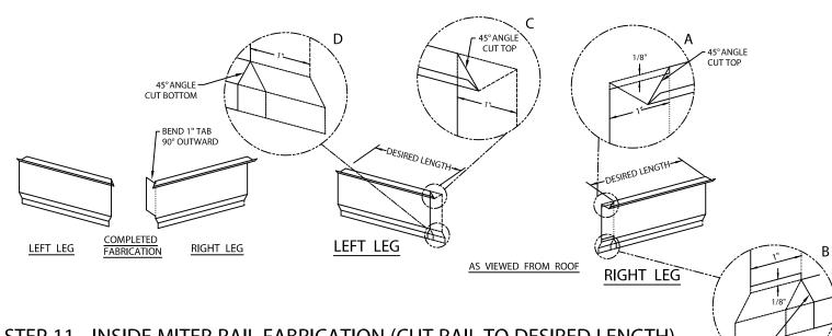
STEP 11 - INSIDE MITER RAIL FABRICATION (CUT RAIL TO DESIRED LENGTH)
