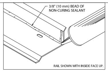
2. Miter & Scupper Base Rail (Preparation) Lay miters and spillout scuppers on deck with outside face down. Be sure aluminum base rail is clean and free of dirt or dust. Apply a heavy 3/8" bead of non-curing sealant to the right angle intersection of the deck flange and back of base rail as shown. Application of sealant is required along the full length of each miter base rail. Apply a similar 3/8" bead of mastic to the flange's left end, as you look at the outside face of the rail section.
