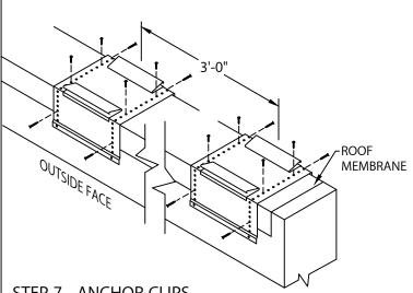
STEP 7 - ANCHOR CLIPS LOCATE OVER ROOFING MEMBRANE AND FASTEN GALVANIZED ANCHOR CLIPS TO WALL AT 3'-0" CENTER WITH PROVIDED FASTENERS AS SHOWN IN DETAIL A
