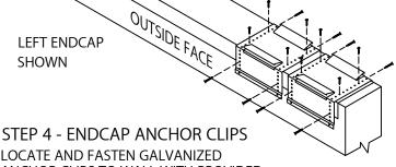
LOCATE AND FASTEN GALVANIZED ANCHOR CLIPS TO WALL WITH PROVIDED FASTENERS FOR SUBSTRATE (SEE DETAIL A).
