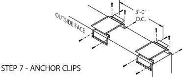
LOCATE AND FASTEN GALVANIZED ANCHOR CLIPS TO WALL AT 3'-0" CENTERS WITH PROVIDED FASTENERS FOR SUBSTRATE (SEE DETAIL A).
