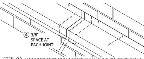
STEP 4- HOOK DRIP EDGE OF EACH BRICK/WALL CAP ONTO CONTINUOUS CLEAT, ROTATE INTO PLACE, AND FASTEN WITH APPROPRIATE FASTENERS. CONTINUE BY INSTALLING BRICK/WALL CAP SECTIONS AND SPLICE PLATES, ALLOWING A 3/8" SPACE AS SHOWN. FIELD CUT AS NECESSARY.
