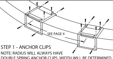
DOUBLE SPRING ANCHOR CLIPS. WIDTH WILL BE DETERMINED BY RADIUS SIZE AND MATERIAL.
