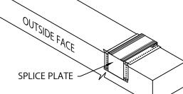
STEP 8 - SPLICE PLATES PLACE SPLICE PLATE ONTO ANCHOR CLIPS AT SPLICE JOINTS, 12'-0" O.C. NOTE: REMOVE RELEASE PAPER FROM SEALANT STRIPS.
