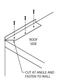
2. OUTSIDE MITER FABRICATION CUT A PIECE OF ELIMINAILER T (ANY LENGTH) ON AN ANGLE. FASTEN TO WALL AT CORNER WITH PROVIDED FASTENERS.
