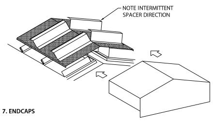
SLIDE ENDCAP ONTO EXPANDED METAL SUPPORT SCREEN. REMOVE PROTECTIVE FILM IMMEDIATELY.
