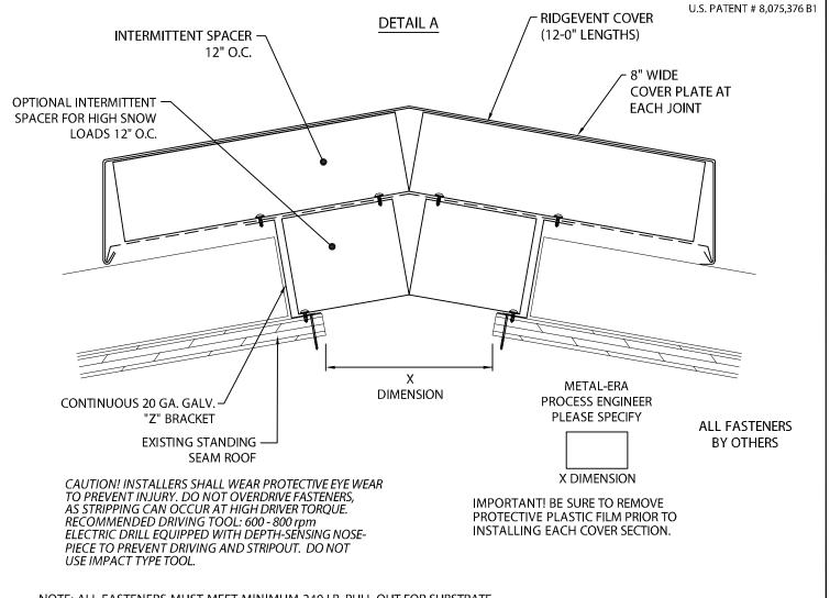
NOTE: ALL FASTENERS MUST MEET MINIMUM 240 LB. PULL-OUT FOR SUBSTRATE.
