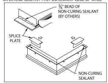
3. ANCHOR BAR MITER SPLICE PLATES APPLY A <sup>3</sup>/<sub>8</sub>" BEAD OF NON-CURING SEALANT (BY OTHERS) TO THE RIGHT ANGLE INTERSECTION OF THE DECK FLANGE AND TO EACH END OF ANCHOR BAR MITER. SLIDE 3<sup>1</sup>/<sub>2</sub>" WIDE SPLICE PLATE HALFWAY ONTO EACH END OF MITER AS SHOWN.
