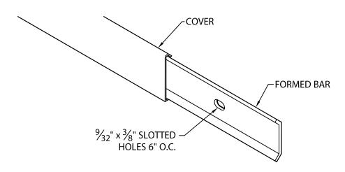
COVER PROVIDED WITH 1" LAP JOINTS SLOTTED FASTENING HOLES  $\frac{9}{32}$ " x  $\frac{3}{8}$ " FURNISHED 6" O.C.
