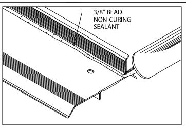
2. Miter & Scupper Anchor Bar (Preparation) Lay miters and spill out scuppers on deck with outside face down. Be sure aluminum anchor bar is clean and free of dirt or dust. Apply a heavy 3/8" bead of non-curing sealant to the right angle intersection of the deck flange and back of anchor bar as shown. Application of sealant is required along the full length of each miter anchor bar.
