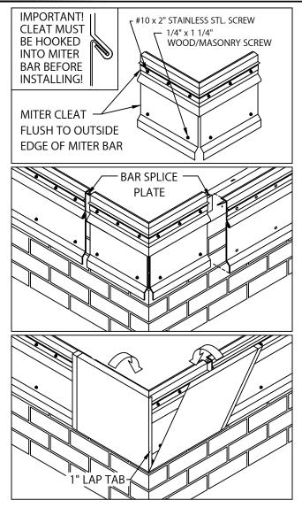
5. MITER BAR & MITER CLEAT INSTALLATION HOOK MITER CLEAT PIECES TO MITER BAR. FLUSH ENDS OF MITER CLEAT PIECE AND MITER BAR. INSTALL MITER ASSEMBLY WITH ONE ANCHOR BAR SPLICE PLATE UNDER EACH END OF MITER BAR. FASTEN THE MITER BAR USING 2" HEX HEAD STAINLESS STEEL FASTENERS. FASTENERS AND DRIVE BITS PROVIDED. NEXT LOCATE AND INSTALL THE SPILLOUTS AND SCUPPERS WITH FASTENERS AND SPLICE PLATES.
