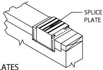
STEP 8 - SPLICE PLATES PLACE SPLICE PLATE ONTO ANCHOR CLIPS AT SPLICE JOINTS, 12'-0" (3.65 m) O.C.
