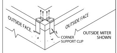
STEP 1 - CORNER SUPPORT CLIPS LOCATE AND FASTEN GALVANIZED CORNER SUPPORT CLIPS TO THE WALL.
