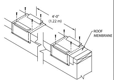
STEP 7 - ANCHOR CLIPS LOCATE AND FASTEN GALVANIZED ANCHOR CLIPS TO WALL AT 4'-0" (1.22 m) CENTERS WITH PROVIDED FASTENERS FOR SUBSTRATE USING THE THIRD FULL TOP HOLE FROM THE BEND (SEE DETAIL A)
