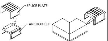
STEP 2 - MITER SPLICE PLATES & ANCHOR CLIPS POSITION THE SPLICE PLATE IN THE CENTER OF THE ANCHOR CLIP. INSTALL THE SPLICE PLATE AND ANCHOR CLIP ASSEMBLY INTO EACH END OF THE CORNER AS SHOWN
