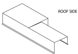
TRANSITIONAL MITER (FOR 2 DIFFERENT WALL WIDTHS) (TAPERED SHOWN)
