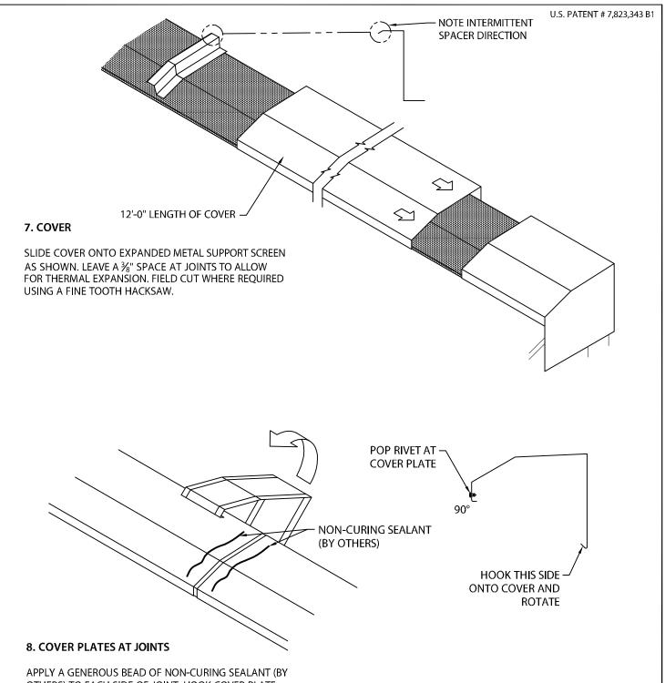
OTHERS) TO EACH SIDE OF JOINT. HOOK COVER PLATE ONTO COVER AT JOINTS AND ROTATE INTO PLACE. POP RIVET INTO COVER PLATE AT ONE SIDE OF THE JOINT (FASTEN SIDE WHICH HAS 90° DRIP ANGLE). THIS WILL PREVENT MIGRATION.
