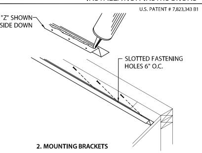
TO PREVENT MOISTURE ENTRY UNDER THE "Z", APPLY A GENEROUS BEAD OF NON-CURING SEALANT TO BOTTOM OF FLANGE. FASTEN BRACKETS TO ROOF AT 6" O.C. WITH APPROPRIATE FASTENERS USING PRE-PUNCHED SLOTTED HOLES. LAP "Z'S" 1".
