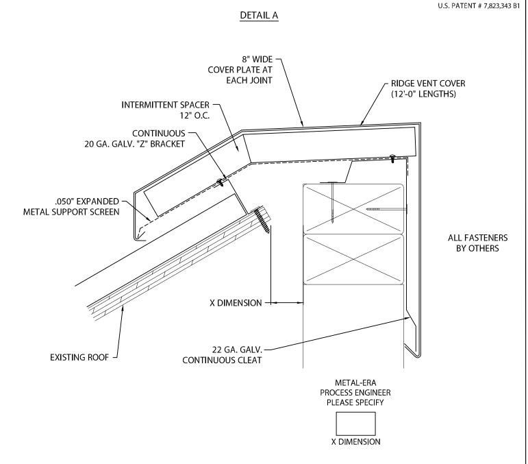
CAUTION! INSTALLERS SHALL WEAR PROTECTIVE EYE WEAR TO PREVENT INJURY. DO NOT OVERDRIVE FASTENERS, AS STRIPPING CAN OCCUR AT HIGH DRIVER TORQUE. RECOMMENDED DRIVING TOOL: 600 - 800 rpm ELECTRIC DRILL EQUIPPED WITH DEPTH-SENSING NOSE-PIECE TO PREVENT DRIVING AND STRIPOUT. DO NOT USE IMPACT TYPE TOOL.
