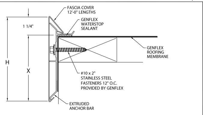
Fascia is to be installed per Specifications and GenFlex's Installation Instructions Dwg. # 22110-2373
