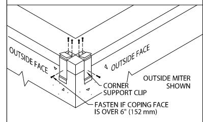
STEP 1 - CORNER SUPPORT CLIPS LOCATE AND FASTEN GALVANIZED CORNER SUPPORT CLIPS TO THE WALL. IF COPING FACE OVER 6" (152 mm), SECURE WITH ADDITIONAL FASTENER AS SHOWN.
