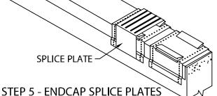
REMOVE RELEASE PAPER FROM TOP OF FACTORY APPLIED SEALANT STRIPS. PLACE SPLICE PLATE ONTO SECOND ANCHOR CLIP AS SHOWN.
