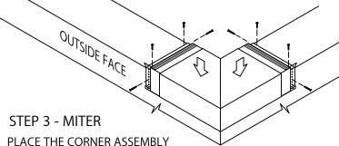
INTO POSITION AND SECURE AT THE EXPOSED EDGE OF THE ANCHOR CLIPS AS PER DETAIL A.
