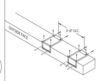
STEP 7 - ANCHOR CLIPS LOCATE OVER MEMBRANE AND FASTEN GALVANIZED ANCHOR CLIPS TO WALL AT 3'-0" CENTER WITH PROVIDED FASTENERS AS SHOWN IN DETAIL A.
