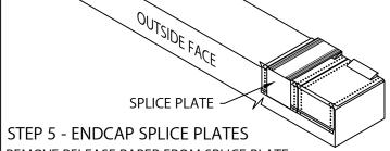
REMOVE RELEASE PAPER FROM SPLICE PLATE SEALANT STRIPS. PLACE SPLICE PLATE ONTO ANCHOR CLIP AS SHOWN.
