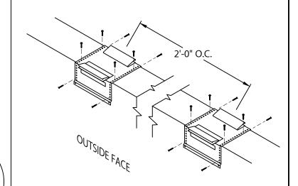
STEP 7 - ANCHOR CLIPS LOCATE AND FASTEN GALVANIZED ANCHOR CLIPS TO WALL AT 2'-0" CENTERS WITH PROVIDED FASTENERS FOR SUBSTRATE (SEE DETAIL A).
