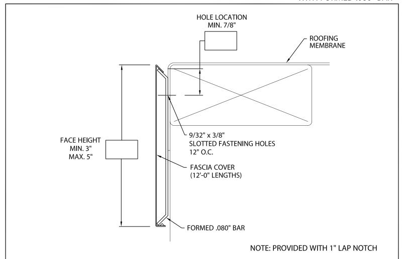
Fascia is to be installed per Specifications and Metal-Era's Installation Instructions Dwg. # 11410-6448
