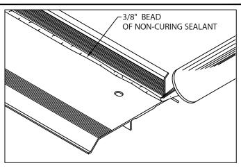
2. Miter & Scupper Anchor Bar (Preparation) Lay miters and scuppers on deck with outside face down. Be sure aluminum anchor bar is clean and free of dirt or dust. Apply a heavy 3/8" bead of non-curing sealant to the right angle inter-section of the deck flange and back of anchor bar as shown. Application of sealant is required along the full length of each miter anchor bar.
