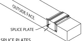
STEP 8 - SPLICE PLATES PLACE SPLICE PLATE ONTO ANCHOR CLIPS AT SPLICE JOINTS
