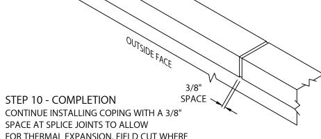
SPACE AT SPLICE JOINTS TO ALLOW FOR THERMAL EXPANSION. FIELD CUT WHERE NECESSARY USING FINE TOOTH HACKSAW OR SNIPS. NOTE: REMOVE PROTECTIVE FILM IMMEDIATELY.
