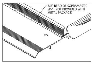
2. Miter & Scupper Anchor Bar (Preparation) Lay miters and spill out scuppers on deck with outside face down. Be sure aluminum anchor bar is clean and free of dirt or dust. Apply a heavy 3/8" bead of SOPRAMASTIC SP-1 (not provided with metal package to the right angle intersection of the deck flange and back of anchor bar as shown. Application of sealant is required along the full length of each miter anchor bar.
